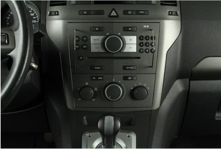
1. Unlock the OE radio with the unlock tool (No. 14) contained in the set. You need to insert two keys.
