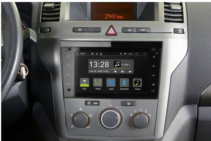
7. Neatly arrange the wires to the side, making room for the Radical device. Carefully slide it into the radio slot. Push back the R-C12OP2 until you hear the clicking sound of the latching mechanism.
