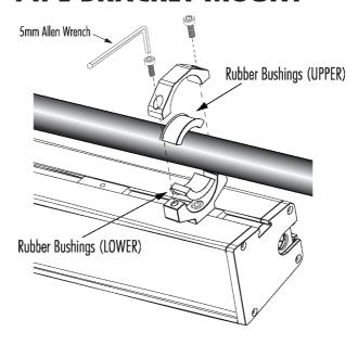
Two rubber bushing sizes are provided. The thinner bushings are for RZR vehicles with 1.75 inch ROPS tubing. The thicker bushings are for ACE and ATV vehicles with 1.5 inch tubing.
