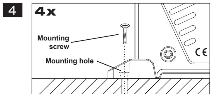
Then uphold the amplifier to the chosen position and fix the screws through the mounting holes into the drilled screwholes.
