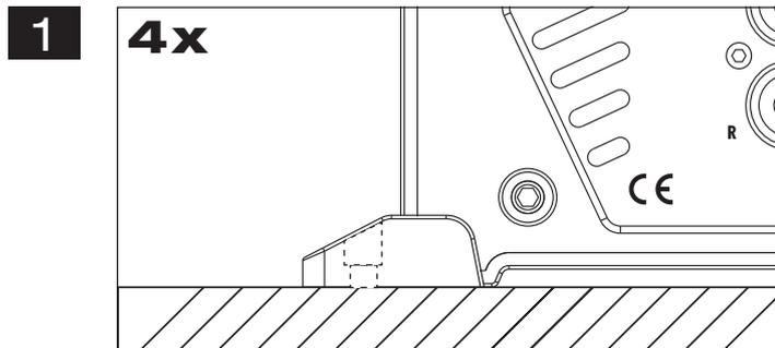
At first you need to find a suitable installation location for the amplifier. Ensure that enough space for the installation of the cables remains and that they will not be bended and have sufficient pull relief.
