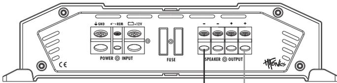
⚠ An additional subwoofer can be connected to the non-occupied speaker outputs. In this case ensure a impedance of 4 - 8 ohms per subwoofer.
