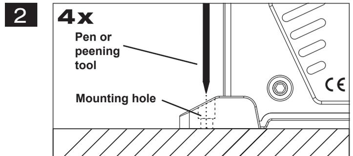
Keep the amplifier at the chosen mounting location in the vehicle. Then mark the four drill holes with an appropriate pen or peening tool through the designated mounting holes at the amplifier.
